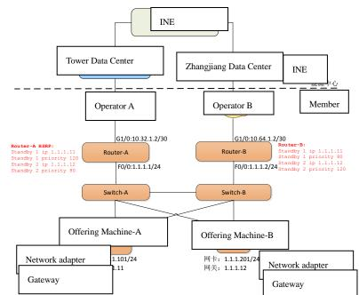
Fig. 5 Network Topology of Offering Machine in Dual Network Adapter Single IP Mode
