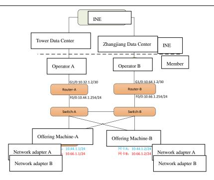
Fig. 4 Network Topology of Offering Machine inmulti-homed Mode
